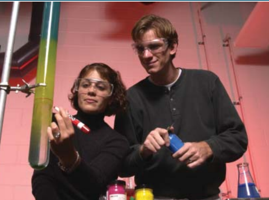
Ph.D. candidates in the EvMM program, Anahita Ahmadi Williamson and Brendan Williamson separate colored xerography toner particles in a density gradient column. They are working with the Xerox Corporation to develop a means of separating waste toner by color so that the toner particles can be recycled. Their preliminary work with black toner illustrated the significant savings and reduced solid waste achieved with toner recycling operations.
